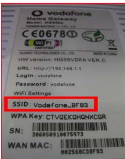
Your own network can be identified as the **SSID** printed on the label on the back of your modem.
